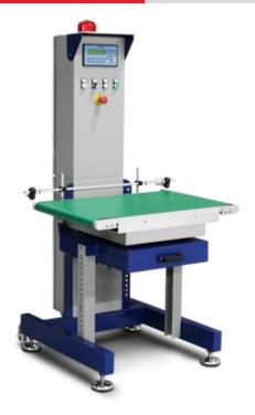
Compact, reliable and accurate +/- weight checking systems. Particularly suitable to be integrated with production and/or shipping conveyor lines for a weight check which guarantees the quality and quantity of the outgoing products. Static or dynamic functioning modes. MID R51 – Start & stop - approvable.
